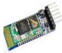
Figure 5: HC-05 Bluetooth Module
